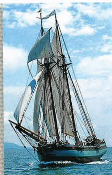
Topsail schooner Pandora, flying sails made by Armando Battaglia of Sailorwear using Oceanus #13 and #10 sailcloth.
